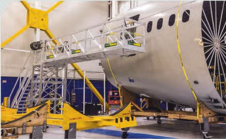
▲ Highly engineered custom cantilever rolling platform for the aeronautical industry
