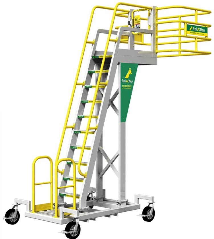
Max height we can make is 13 step. Modified Cantilever Max at 36". Base is Galvanized Steel, upper is mill finish aluminum, yellow powder coat rail, aggressive tread step surface. Unit can be modified adding Forklift channels to assist with movement of the platform at your site.
